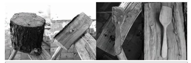
Figure 2: From left to right: A) A sawn section of the log is called a bolt. B) The cleft bolt produces several billets. C) The billet is axed out into the rough spoon outline or blank. D) The blank is refined with the knives into a usable spoon.
